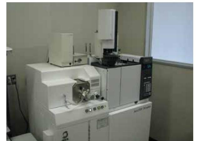
Gas chromatograph time-of-flight mass spectrometer
