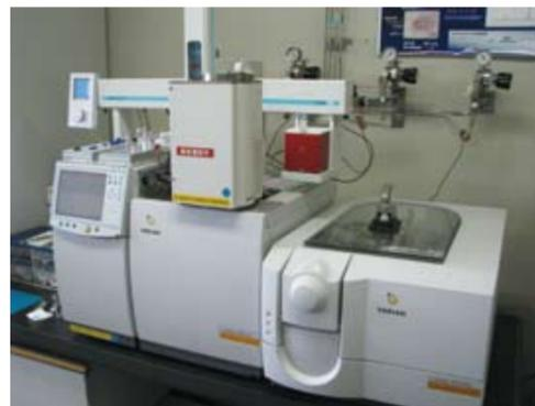
Pyrolysis gas chromatograph mass spectrometer
